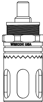
WES296-SL-S Microstop with Ø 1/4" Standard Shaft
